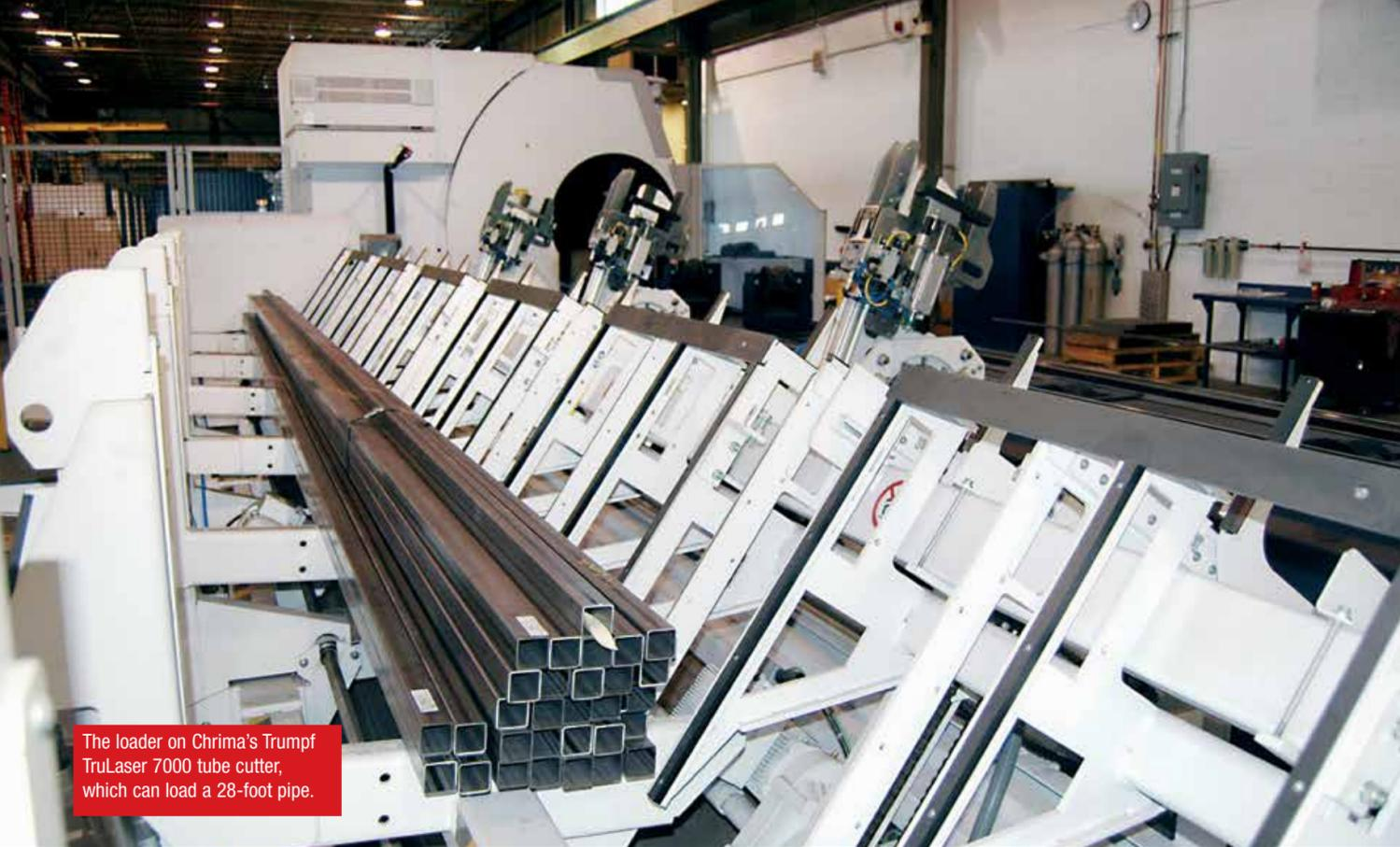
The loader on Chrima's Trumpf TruLaser 7000 tube cutter, which can load a 28-foot pipe.
